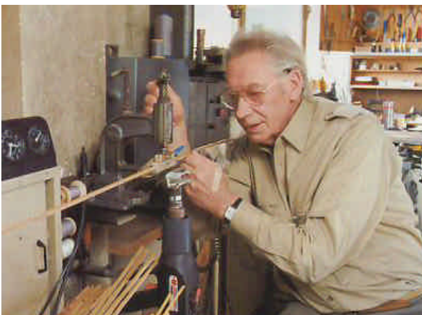
Brunner splitting a culm next to a 60° beveller built in 1964 and during node treatment.
