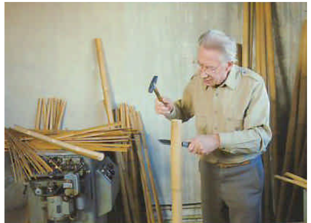
Brunner splitting a culm next to a 60° beveller built in 1964 and during node treatment.
