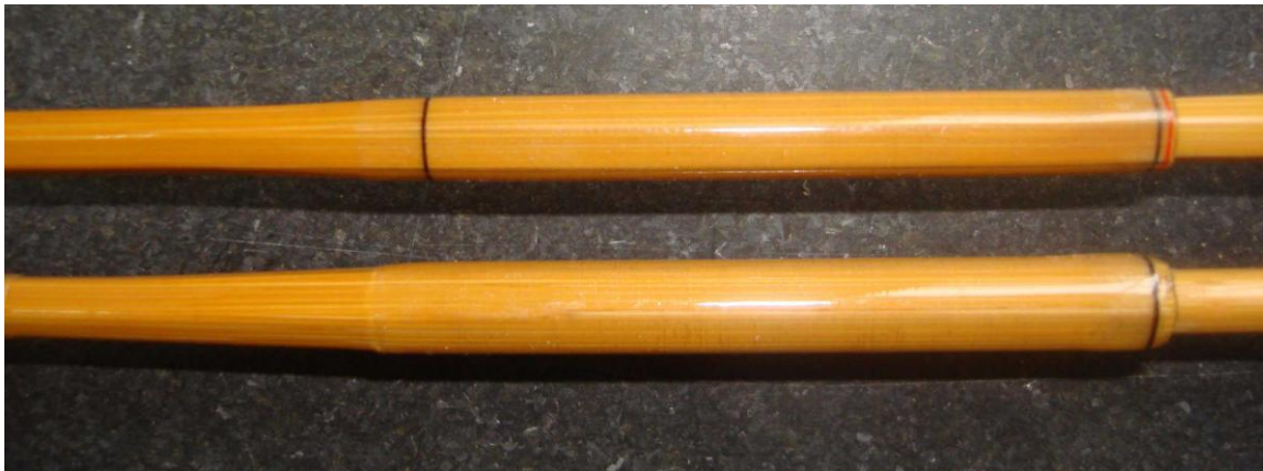
Comparison between a Streamlined ferrule (above) and a normal ferrule (below) Photo and rods by Philipp Sicher
