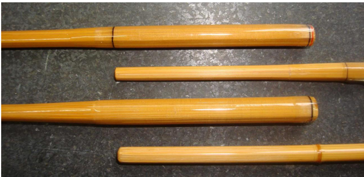
Comparison between a Streamlined ferrule (above) and a normal ferrule (below) Photo and rods by Philipp Sicher
