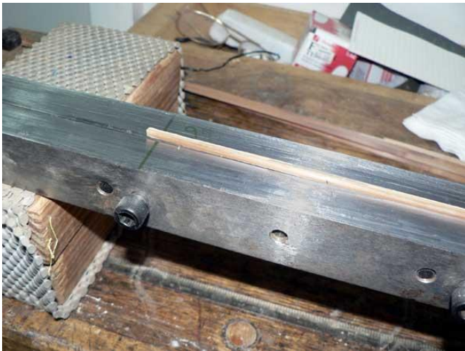
Look closely and you can see that the enamel side is towards you, the pith apex side of the strip away from you in the planing forms
