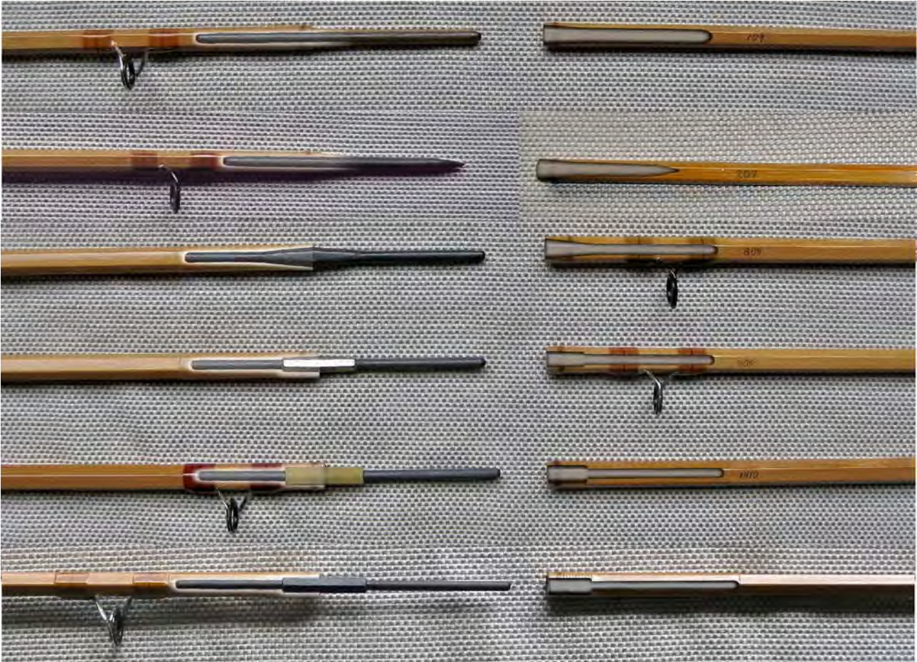
Figure 3. Internal structure of the ferrules.
