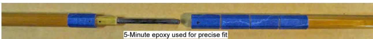
Figure 5. Preparation for fitting spigot to socket.
