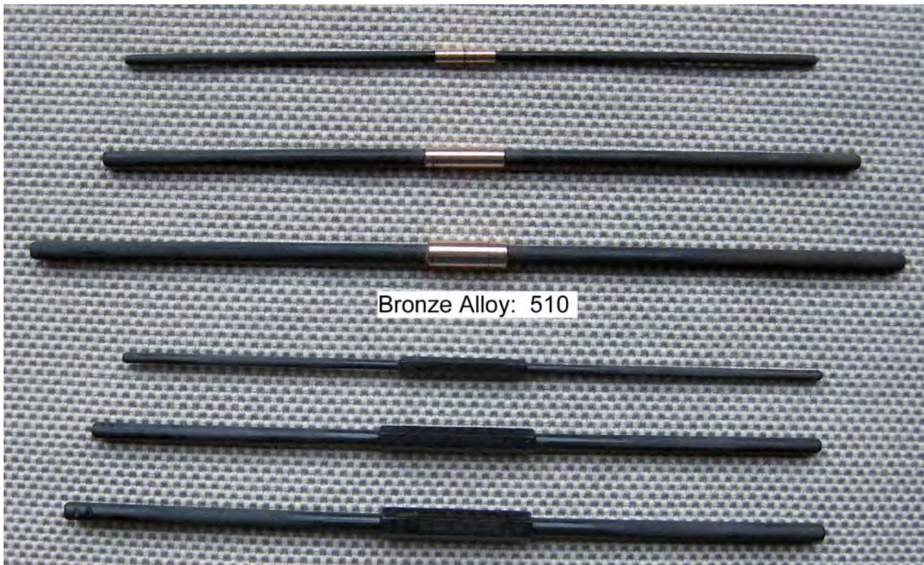
Figure 6. Spigot generation five. Glued with UHU Endfest 300; flats cut after gluing. Bronze tube is about 0.1" (2 mm) shorter than hexagonal plastic sleeve.
