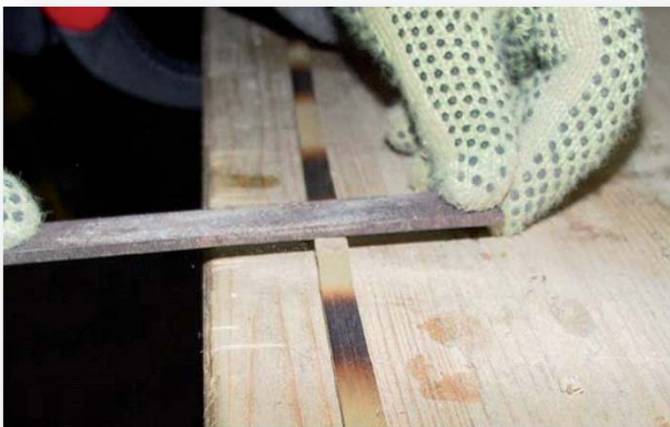
Filing as the removal of the external bump of the node and the Pressing
