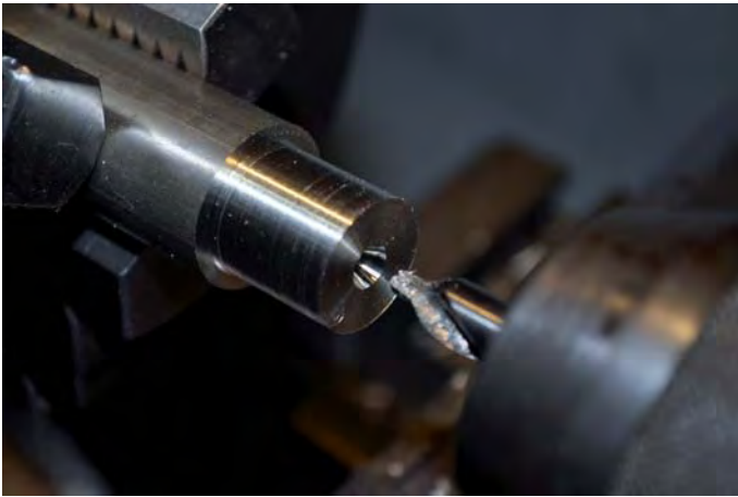
3) Centre hole drilling.
