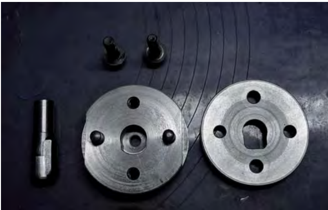
11) Components of the die, from left, punch, mould, counter-mould.
