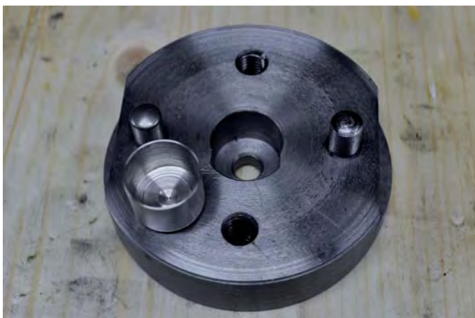
10) Butt cap ready to be punched.
