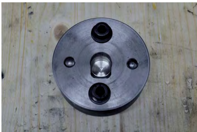
17) Close the mould, the cap and the counter-mould by tightening the screw.
