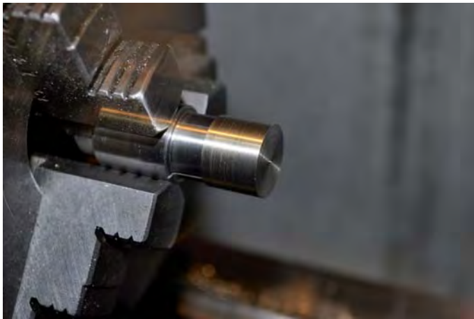
8) With the cap on the expandable chuck, face off to remove the little nipple caused by the parting tool.
