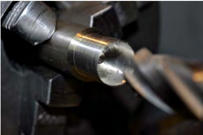
5) End-milling the bottom.
