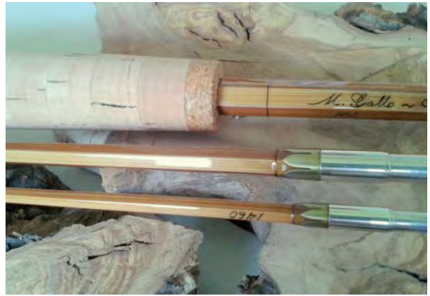
MICHELE GALLO (TRANSPARENT TYING ON STEP-DOWN FERRULES)
