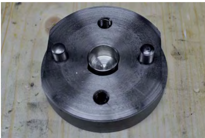
16) Preparing for the punching of the pocket. Insert the cap in the mould.
