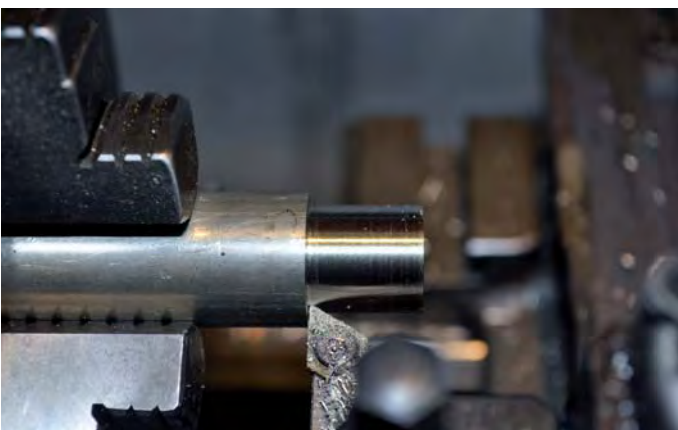
2) Rough turning and external finishing.
