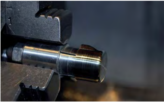
22) Finish the surfaces with sandpaper.
