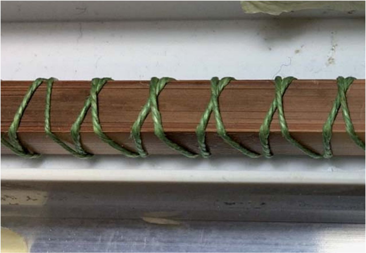
Fig. 5- Final double wrappings with tying cord.
