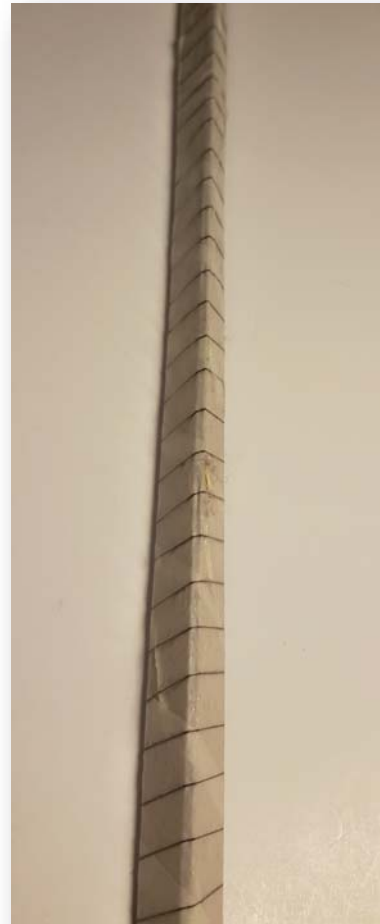
FIGURE 2: measurement of bending (rod with spiral wraps).
