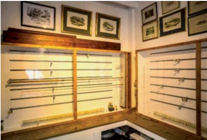
The varnishing cabinets in which whippings are varnished.
