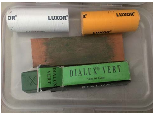
Fig.3. The green strop is 0.7 micron, Chrome oxide, the white is 0.3 microns and the yellow is 0.1 microns, both Aluminum oxide.
