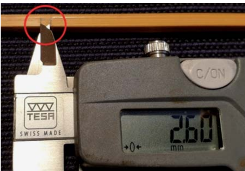
Measurement of male slide
