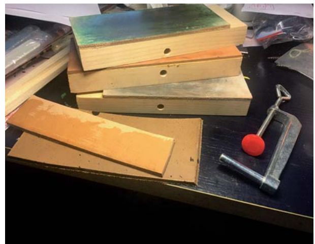
Fig. 7. Some leather strops, two pieces of hard cowhide, and the bar C-clamp to fasten
