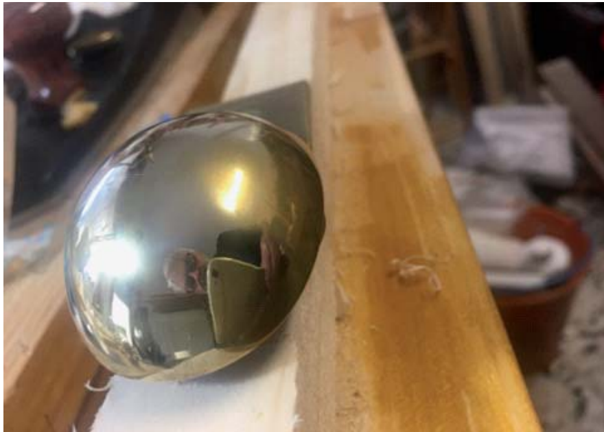
Fig. 5. Hazy image due to poor polishing. The haze is generated by the scattering due to residual surface roughness.
