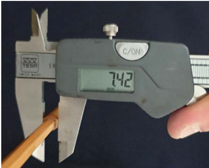
O.D. of the female measured "face to face" with the inserted male taken at the opening
