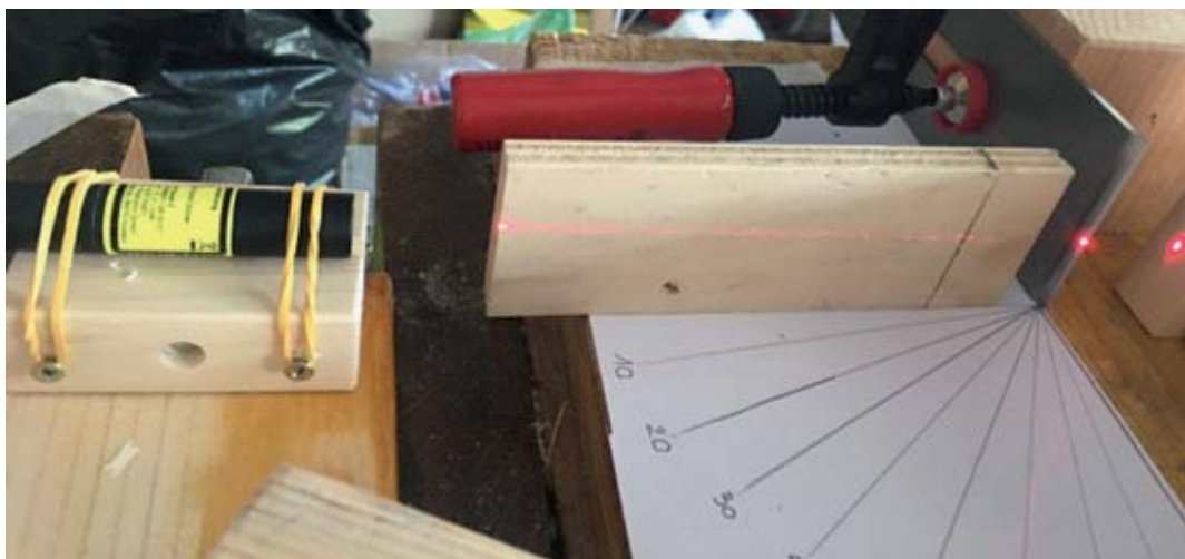
Fig.8. Side view. At left the laser pointer and its mounting block. The beam goes from left to right, and to try to make evident the beam, a plywood panel is placed parallel to the beam so that it grazes the panel (see the weak red line at mid height). The beam hits the blade partially. Notice the spot onto the beam stop further away from the blade. Finally, a crude protractor measures the reflected angle direction (see next image).
