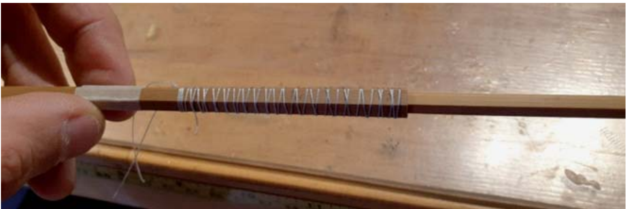
Wrapping a hex TBF ferrule during the gluing of the tip
